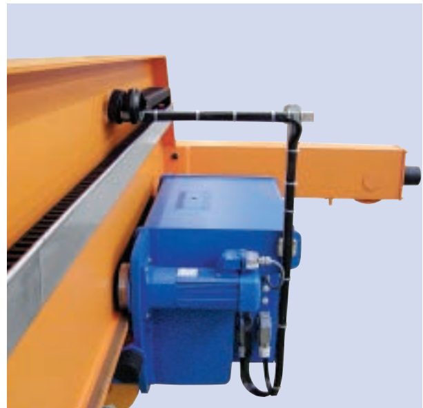
Signal transmission and power supply to hoist
